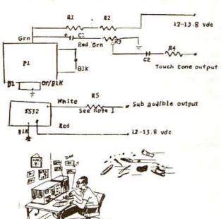
Note: The value of R5 has to be determined by experimentation, and a good way is to use a 1 meg pot in series with output and vary it for best operation. Different sets take different values, with my Tempo VHF S-1, I wound up with a half megohm there, as I used a 470k ohm 10%.
