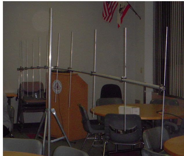
Twelve element, 14.5 db gain Yagi antenna.
