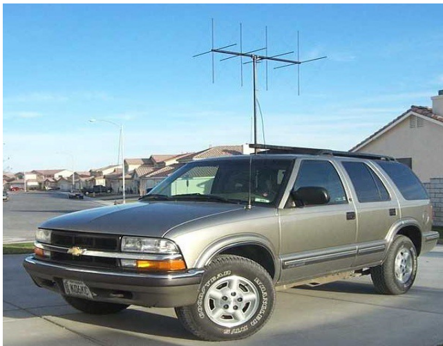
T-hunting Vehicle configured with a quad that can be manipulated from the inside.
