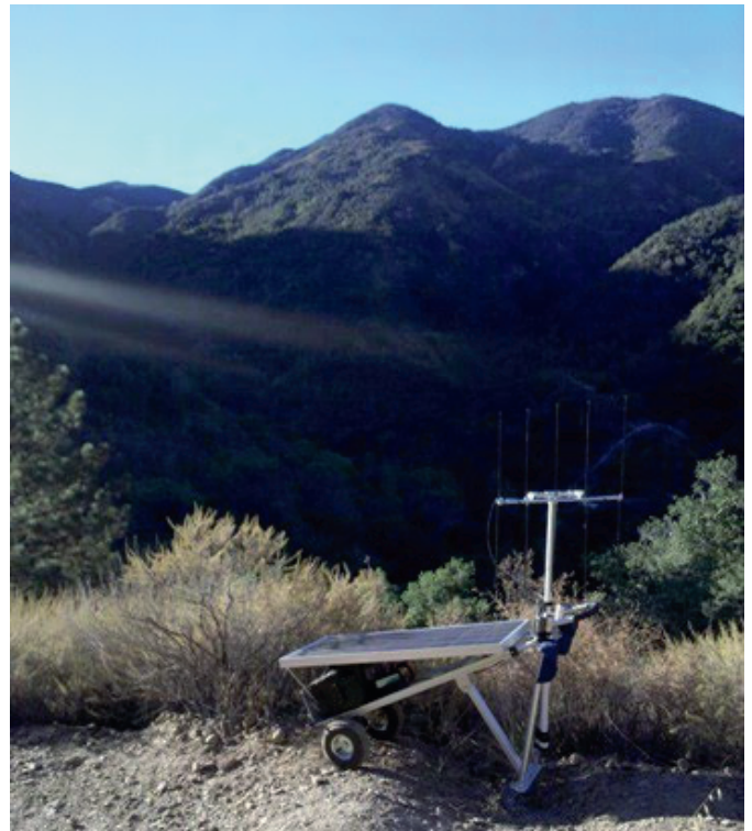
50 watt solar powered repeater deployed and working.
